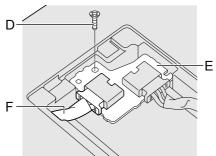
6. Pull out the built-in bridge battery with the sheet cover.
